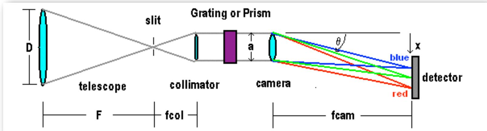
Note: The slit mainly serves to isolate light from the target and is sometimes omitted.
