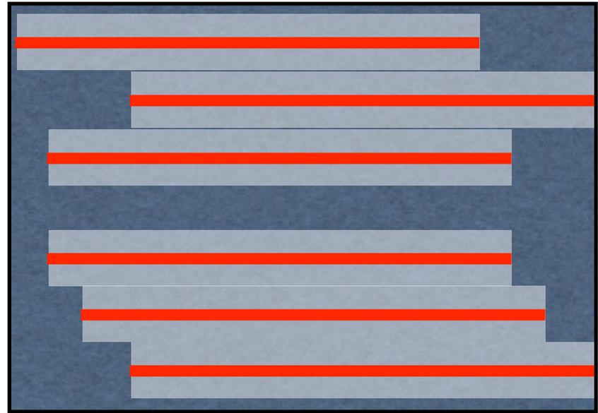
Slit masks can be fabricated for each case (typically by cutting slits in a metal plate).
