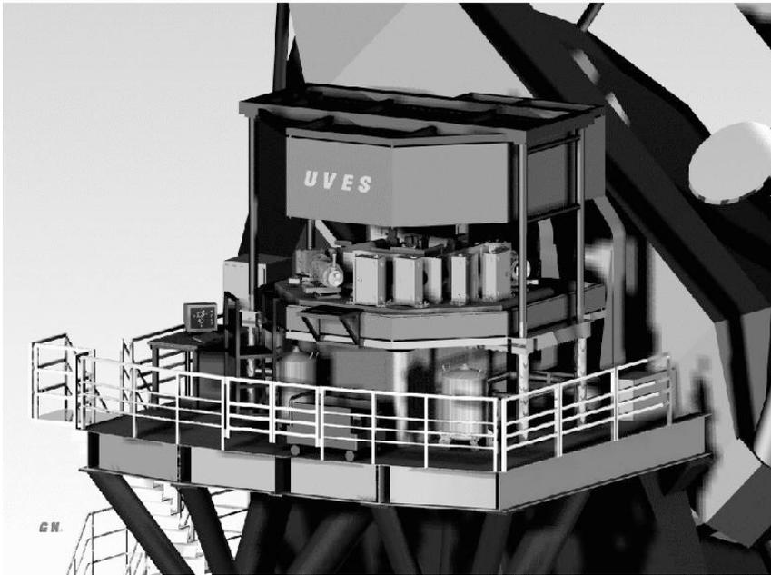
Figure 1.1: The UVES spectrograph on the Nasmyth B platform of VLT Unit Telescope #2 (3D CAD view).
