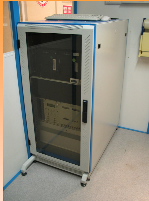
Mark4 Formatter + Mark5A recorder
