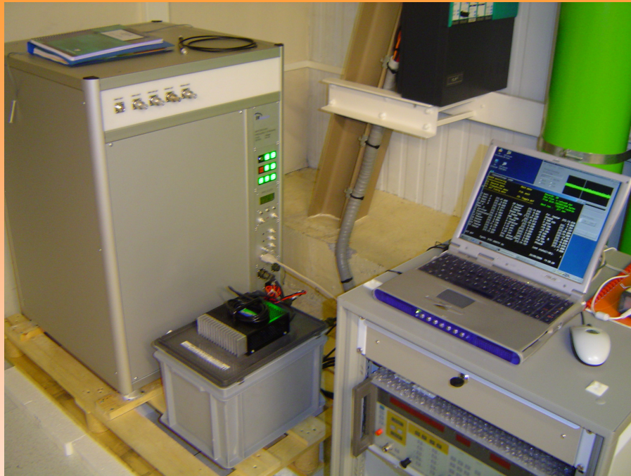
EFOS-38 maser (T4Science), with low phase noise quartz
